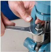
The gap between the spring stack cover and the gland plate is pre-set to 1 mm on initial installation.
