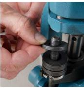
Live-loading systems can be quickly fitted to an existing valve. The required spring loading etc. is calculated by our application engineers from your site measurements.
