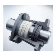
Insert more rings into the stuffing box making sure that each cut joint is at  $90^\circ$  to the previous ring joint. Rings should be added until the gland projects (for guidance) into stuffing box compartment by at least 1/4 (for valves) or approx. 1/2 (for pumps) of the packing width "s". Press the rings home with the gland and tighten the nuts hand-tight. If there is a lantern ring, check that it is correctly positioned in relation to the inlet connection after the gland has been tightened.
