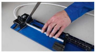
EagleBurgmann packing cutters (9612, 9616) ensure precisely cut rings. If no cutter is available, proceed as follows, The cutting length L is dependent on the shaft diameter d and the packing width s according to the following formula:
